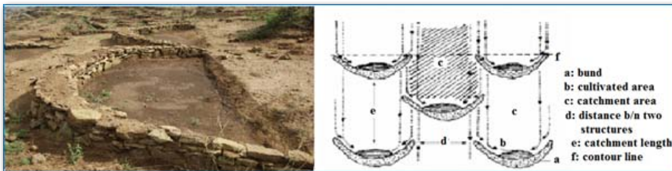
Fig 3.4 Design and construction of semi-circular bunds
